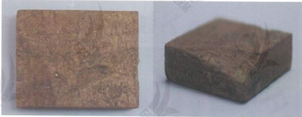
Figure 3 Rubberwood samples after 4 weeks of termite test. (Left) Top view. (Right) Side view.
